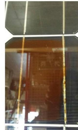
2 Solder bond failure of both cell interconnects
